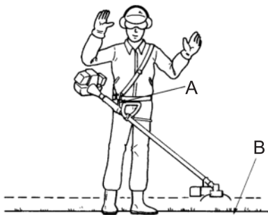
Balance tool for a level plane of cutting head rotation
